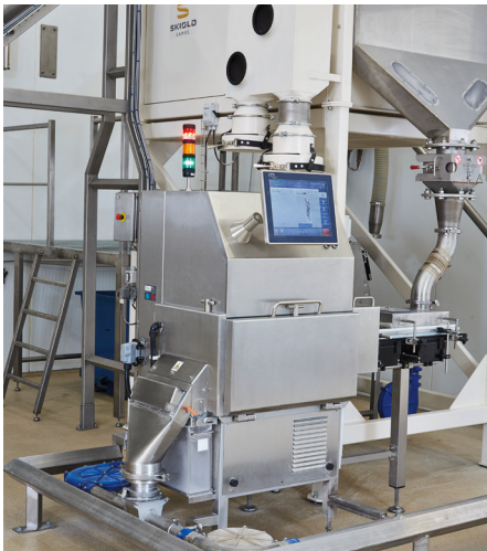
X-ray scanner at DANRICE. The product arrives on the conveyor belt via a pipe system (right) and is conveyed through the scanner
