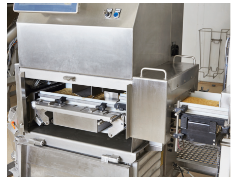
Product flow with system open. Due to the various planes inside the X-ray scanner, radiation cannot escape via the transport openings and the unit is safe during operation
