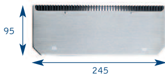
Controller Front Elevation
