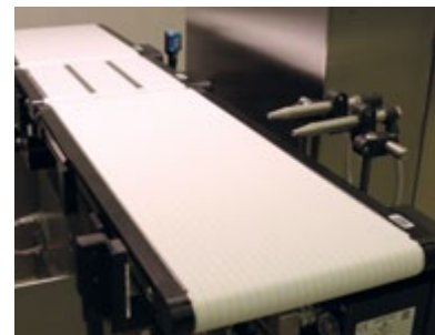
Air blast nozzle for secure ejection of under or overweight products
